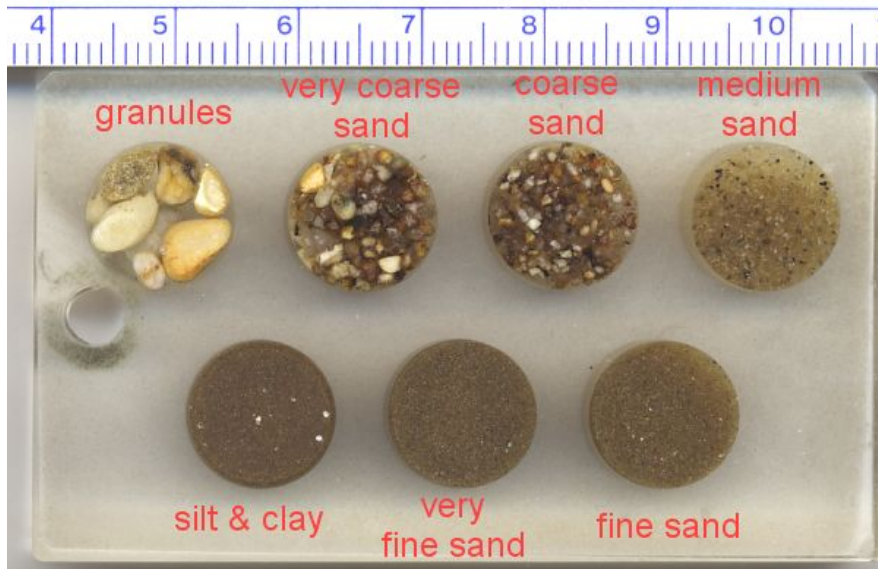
Figure 5: Example of sediment comparator card that could be used to assist observers in distinguishing sediment types (silt vs. sand). Image from: http://www.virtual-geology.info/sediments-and-strata/grainsize.html
